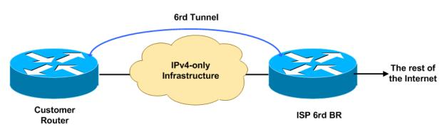
The Customer Router in the diagram is our Customer Router in our network. And the ISP 6rd BR capability will be configured on our autonomous system's Border Router.
