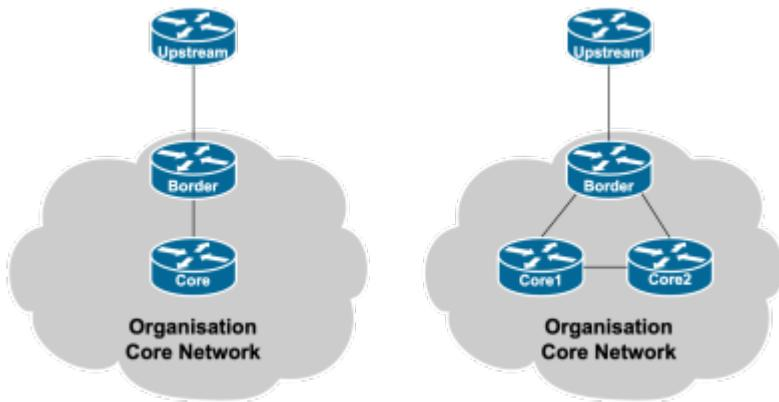
It is recommended to separate the router that has the upstream connection from the core of the network, for the security of having a clear demarcation point, and so that specific border functions don't overload the core devices in the network.
