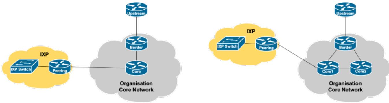
In more sophisticated cases, especially where the IXP is providing a significant portion of the organisation's traffic, a second peering router might be procured, to provide not only link redundancy but also router redundancy. This second/redundant infrastructure will likely only be deployed a bit further down the track, after gaining sufficient operational experience of traffic levels and infrastructure reliability. The diagram below shows this scenario:
