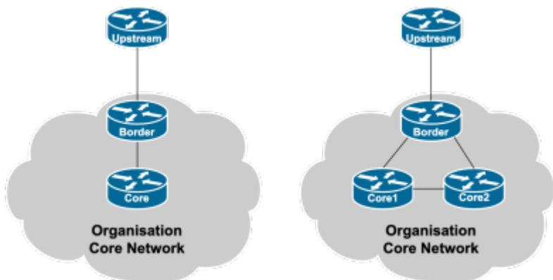
It is recommended to separate the router that has the upstream connection from the core of the network, for the security of having a clear demarcation point, and so that specific border functions don't overload the core devices in the network.
