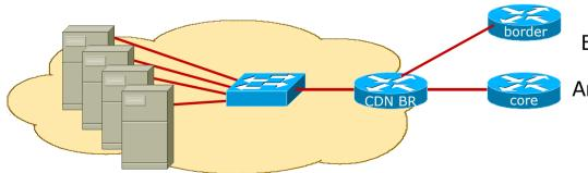
Connection to Network Operator Border Router (Transit/Cache-Fill)
