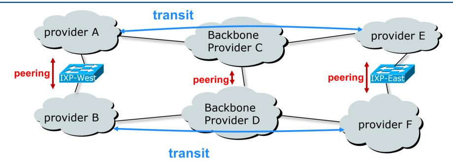
A and B peer for free, but need transit arrangements with C and D to get packets to/from E and F
