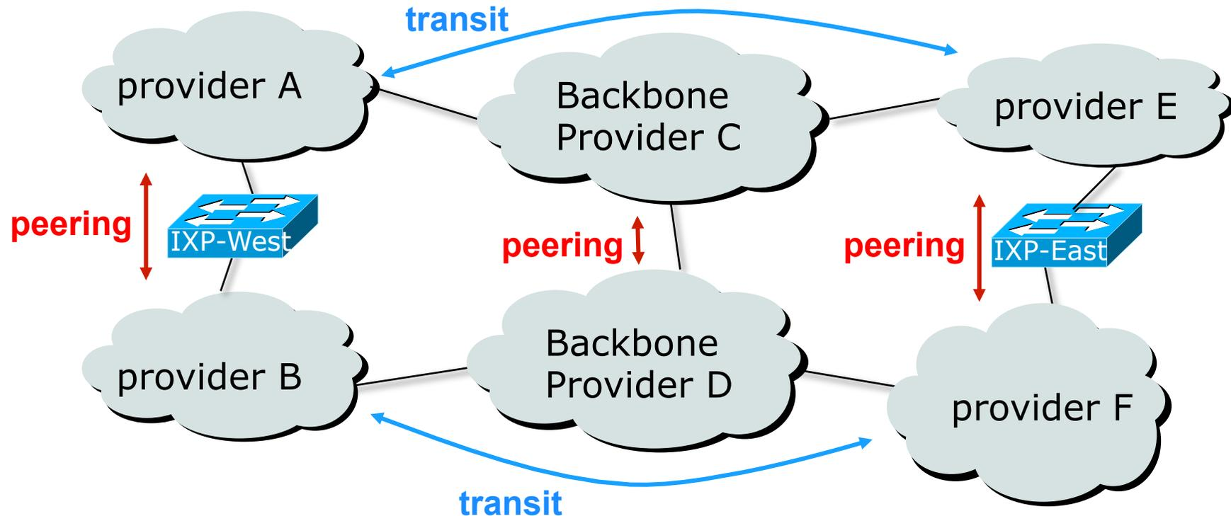
A and B peer for free, but need transit arrangements with C and D to get packets to/from E and F
