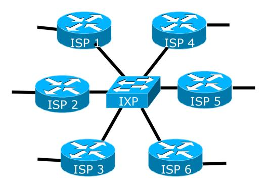
Each of these represents a border router in a different autonomous system
