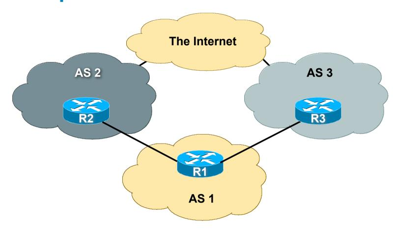
Symptom: AS1 is loadsharing between its upstreams, but the traffic load swings randomly between AS2 and AS3
