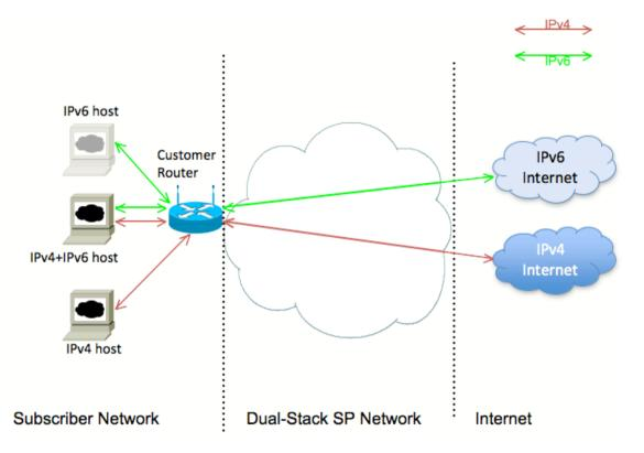
The original transition scenario, but dependent on: IPv6 being available all the way to the consumer Sufficient IPv4 address space for the consumer
