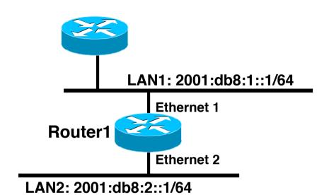
Dual IPv4/IPv6 configuration - note single-topology command —
