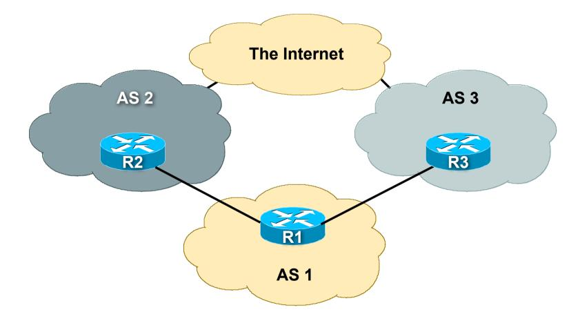
Symptom: AS1 is loadsharing between its upstreams, but the traffic load swings randomly between AS2 and AS3
