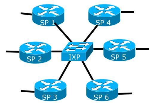
Each of these represents a border router of a different network operator
