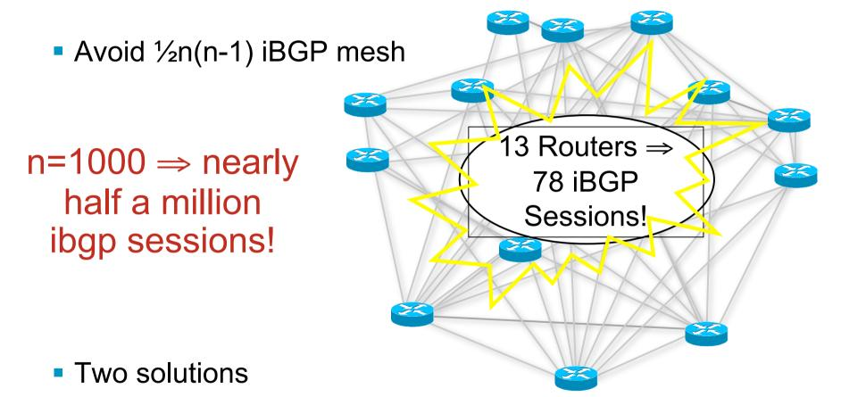
Route reflector – simpler to deploy and run
