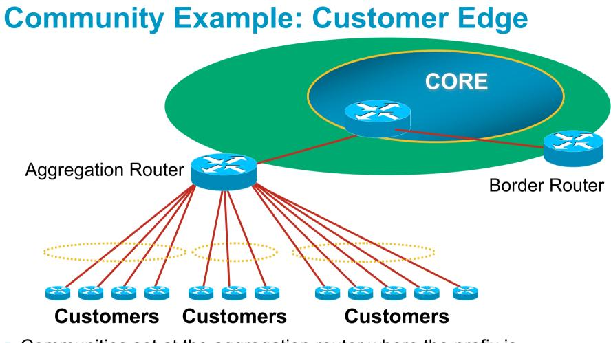
Communities set at the aggregation router where the prefix is injected into the ISP's iBGP
