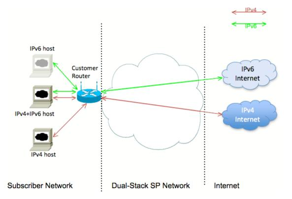
The original transition scenario, but dependent on: IPv6 being available all the way to the consumer Sufficient IPv4 address space for the consumer
