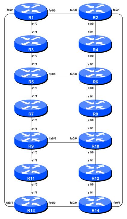
Figure 1 – ISP Lab Basic Configuration
